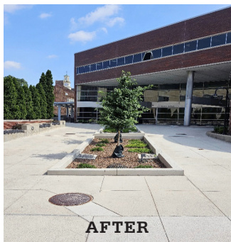
Attractive landscape planters double as stormwater spillways to capture excess rainwater.
